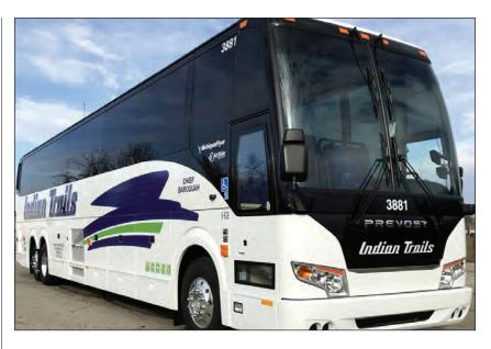
kneeling suspension to help passengers get on or off. The coaches exceed EPA standards with engine technology that cuts exhaust pollutants to near zero while achieving 240 passenger miles per gallon.
