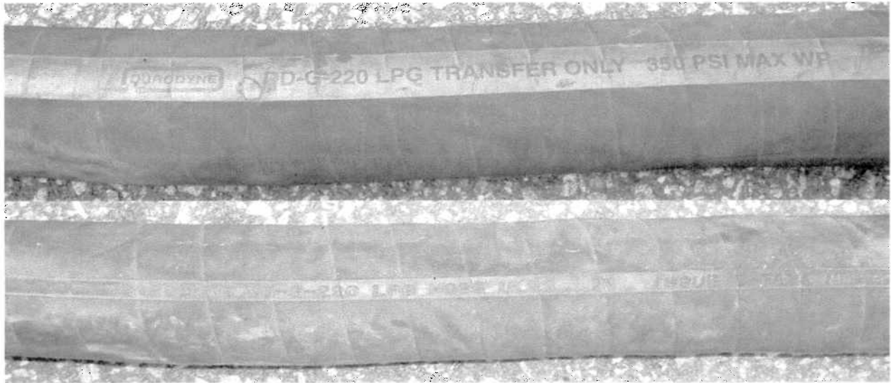
Figure 1: Example of LPG-Use Only Hose Marking
