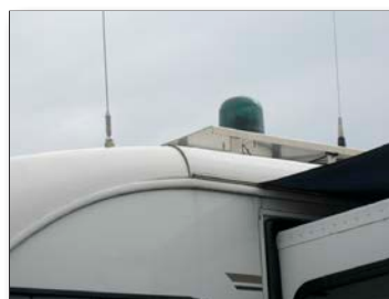
Figure 4.13 — Green warning lights are commonly used to designate a mobile Command Post vehicle. (Photo/Mike Wieder)
