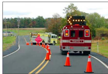
Figure 7.30 — Some fire apparatus are equipped with lighted directional arrow or message signs. (Photo/Bob Esposito, Pennsylvania)
