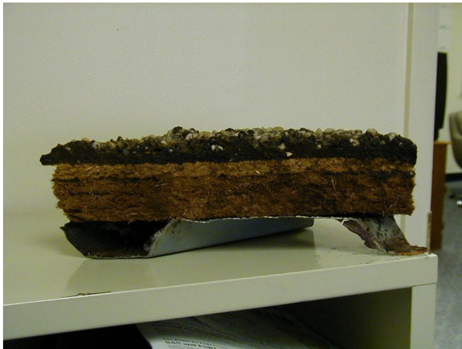
The sample roof section above was cut using a carbide-tip chainsaw.
