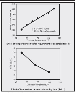
result in plastic shrinkage before concrete sets or early-age drying shrinkage cracking. The evaporation rate removes surface water necessary for hydration unless proper curing methods are employed. Thermal cracking may result from rapid changes in temperature, such as when concrete slabs or walls are placed on a hot day followed by a cool night. High temperature also accelerates cement hydration and contributes to the potential for thermal cracking in thicker concrete sections.
