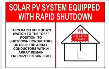
Label for PV Systems that Shut Down Down the Conductors Leaving the Array Only.
