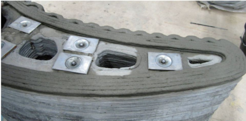
Functional voids and customized, threaded rebar for post-tensioning
