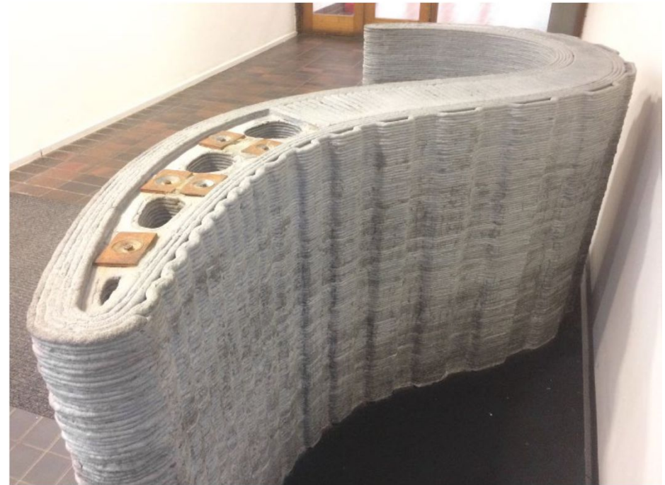
Example of element manufactured using fine filament ("endless loop") deposition method.
