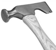
**Drywall hammer.** The serrated face of this appropriately named hammer gives you a better grip on the nail when installing drywall. You can use its hatchet-shaped back for cutting drywall.
