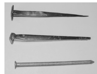
Handmade nail (top) Cut nail (middle) Wire nail (bottom)
