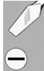
**Slot head screwdriver (Flathead/regular screwdriver).** A slot head screwdriver consists of a single, flat blade that fits in the single slot of traditional screws. You find these everywhere, though the practice of using screws with slotted drives is on the decline because the screwdriver slips out of the slot, particularly when you are applying heavy torque to really tighten down (or loosen, for that matter) these types of screws.
