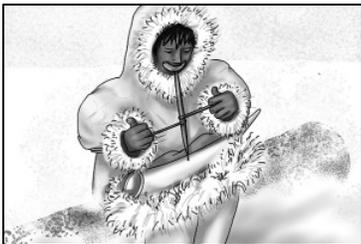
The first step forward in drilling was the strap drill, which had a leather cord wrapped around the shaft of a stick. By pulling the cord back and forth, the stone bit at the end of the stick could be rotated at a higher speed, making it more effective.
