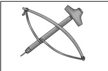
After the strap drill came the bow drill, which first appeared in Egypt over 6,000 years ago. The bow drill consisted of the two ends of leather from a strap drill attached to a bow. This made it easier to move back and forth, rotating the drill. The bow drill could be rotated faster than the strap drill, speeding up the drilling process.
