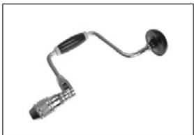
At the end of the 19th century, good quality cheap steel allowed much stronger braces to be made. With the advances in manufacturing accuracy at the time, more complex parts could be made. This led to improved chuck designs and the invention of the ratchet mechanism that would be used on some braces and hand drills.
