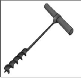
During Roman times, the auger drill became popular. The auger was a metal corkscrew-like drill with two wooden handles at the top, giving it a 'T' shape. It was better suited to drilling wider holes than other drills that required several people to turn, so was used to drill very large diameter holes. Auger shaped drill bits are still used to this day in modern drills for drilling larger diameter holes into wood.
