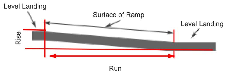
**Components of a Single Ramp Run**
