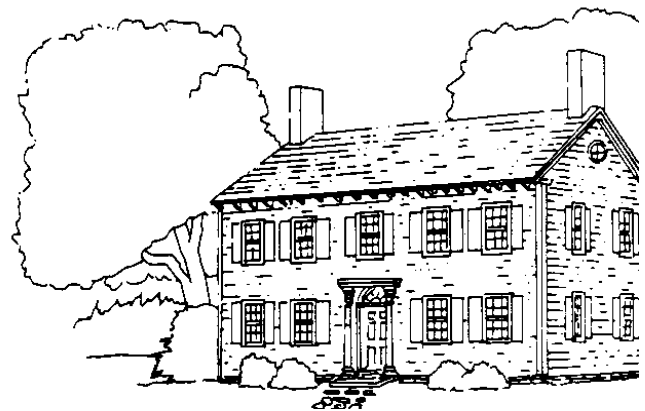
Gabled roof, cornice and fan light
